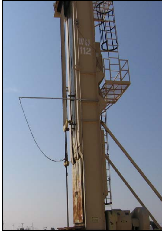
Figure F-1. Recommended Load Cell Cable Routing
